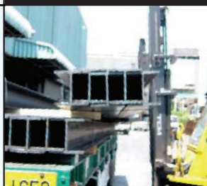
Check the carrying weight of the forklift before lifting and carry at the middle of bundle
